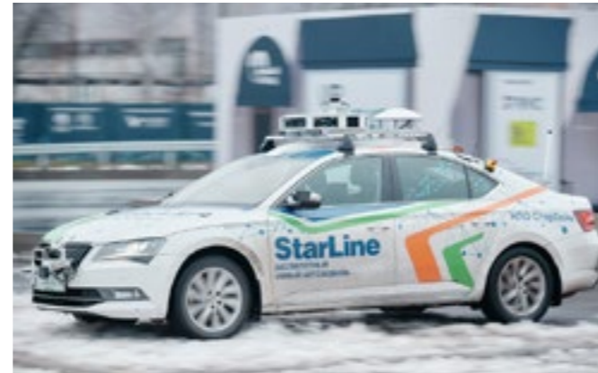
The sensors we selected have different physical principles. This ensures their stable operation in various weather conditions, like rain, snow or fog.
